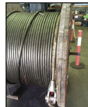
Figure 7. The triple-armoured umbilical of choice providing fiber optics, 240V, and lifting capabilities.
