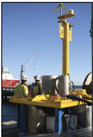
Figure 3. The skid that sits within the outer skin of the DPP
