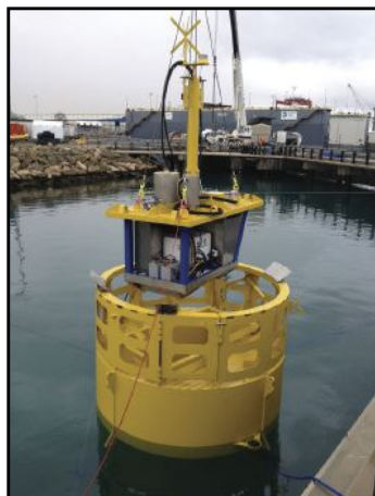
Figure 4. The two parts of the DPP being aligned (can be deployed as one or two parts depending on vessel)
